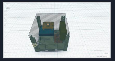
Basic CubeSat plan. Components should include most acrylic pieces, corner rails, and hardware that interacts with the pi. Simple, elegant design, prioritizing ease of access to hardware and lasting battery life.
